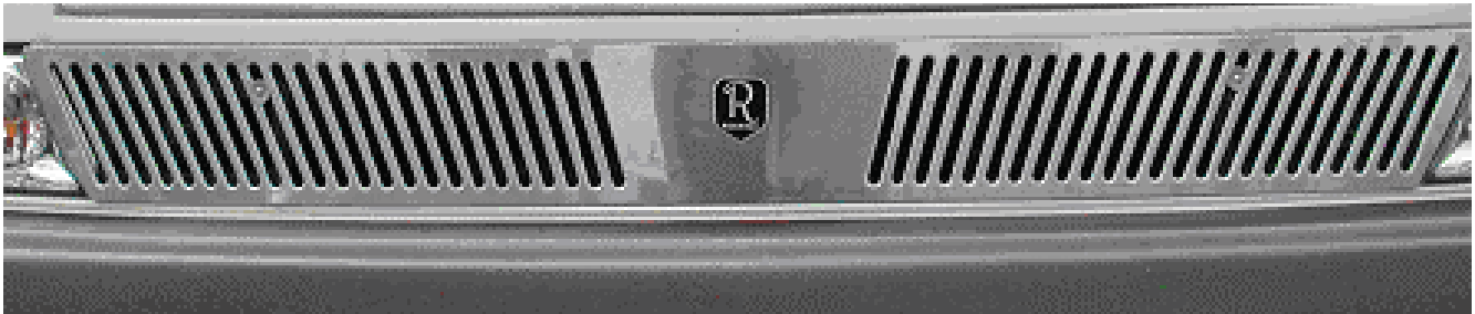
Illustration 3: Front of Vehicle with Intake Ducts Fitted (Example)
